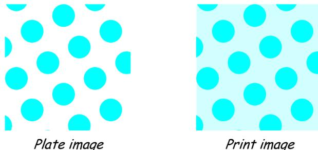
This optical dot gain is a second component to tone value increase that goes beyond the size of the dots. A planimeter will not be affected by optical dot gain, but a densitometer will.
