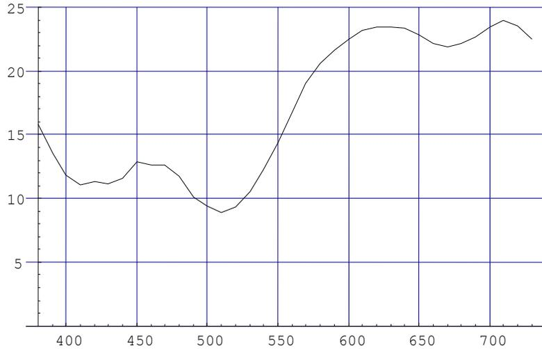
case, this shows that the amount of optical dot gain depends upon wavelength. Curiously, the optical dot gain is apparently related to the reflectance of the ink. There appears to be more optical dot gain where the reflectance of the solid is lowest.
