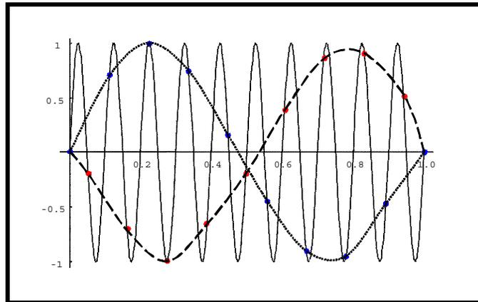
**Figure 5: Illustration of Sampling a Sine Wave**
