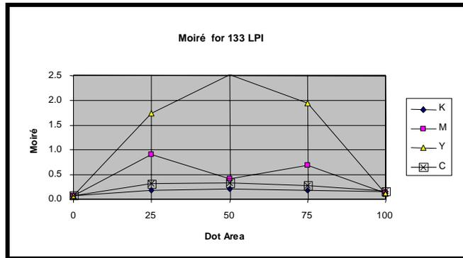
**Figure 8: Measured Moiré for 133 LPI Patches**
