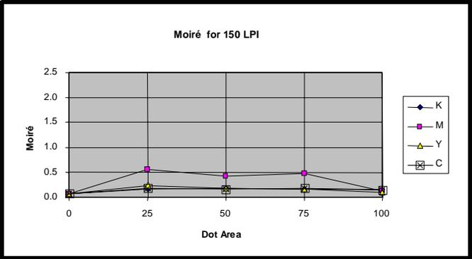
**Figure 9: Measured moiré for 150 LPI patches**
