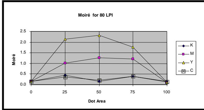
**Figure 6: Measured Moiré for 80 LPI Patches**
