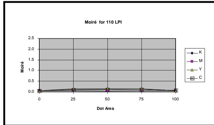
**Figure 14: Affect of Optimized Filter on 110 LPI**
