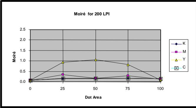
**Figure 10: Measured Moiré for 200 LPI Patches**
